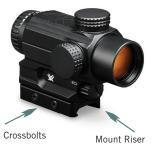
2. Check that the mount fully engages the base, press the Spitfire down and forward, then tighten the base crossbolts.
