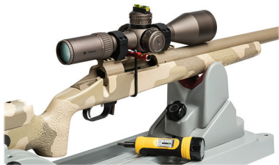
Using bubble levels to square the riflescope to the base.
