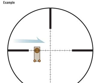
9.5 MOA reticle correction for a target moving 3 mph at a distance of 800 yards. No wind. Total bullet time of flight from moment of trigger pull is 1.5 seconds during which a target travels 6.6 feet. Elevation already dialed into turret.
