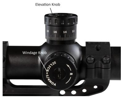
The TS-20X features 1/4 MOA or 1/10 MIL clicks on both the elevation and windage knobs. The click value specific to your optic is engraved on the knob. The elevation and windage knobs feature a directional arrow which indicates the direction your impact is moving when the knob is adjusted.
