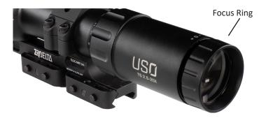
The focus ring is used to focus the reticle. Focus prescription ranges from +2 to -3. Do not use the focus ring to adjust the sight picture or to adjust for parallax.
