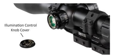
To remove/replace the battery, turn the illumination control knob cap counter clockwise until battery is exposed. Remove the old battery. Insert a CR2032 battery with the positive side (+) facing outward. To secure the battery in place, attach the illumination control knob cap by turning it clockwise.
