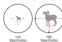
Second focal plane (SFP) reticles sit behind the erector, resulting in reticle subtensions that are calibrated to a specific magnification. Unlike FFP reticles, second focal plane reticles appear constant in size regardless of the magnification.
