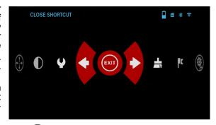
Use the LEFT & RIGHT buttons to move between functions, except with the group of ON/OFF switches (WiFi, Bluetooth, Ballistic Calculator, RAV), use the Scroll Wheel or Keypad buttons between switches.
