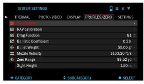
Proceed to Zero the Reticle. Press the OK button to select Zero Reticle. You will see on your screen a cross hair reticle. While keeping the gun as steady as possible, fire a round. Use the key pad and scroll wheel to move the Red cross hair to the point of impact. While keeping
