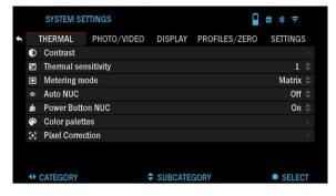
METERING MODE — The Center mode tells the sensor to concentrate on the heat signature in the center of the field of view and ignoring the background.
