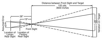
The diagram above shows how a longer "Sight Radius" affects the accuracy of your shooting. An average increase of 11" in "Sight Radius" translates into 32% greater inherent accuracy at 100 yards. This greater inherent accuracy is proportional to the target range, i.e., 32% at 100 yards, 64% at 200 yards, 128% at 300 yards etc. It is easy to understand why all match target rifles use a rear aperture sight mounted as far to the rear as possible.
