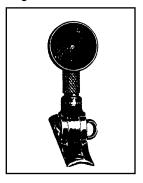
merely of screws flattened on the end with a small hole drilled in this flat portion. The elevation was obtained by turning this screw in the stock, one-half rotation giving an elevation equal to one-half the pitch of the thread.
