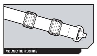
To connect the QD Sling Swivel to the sling, run the end of the MS1 through the QD Sling Swivel and then back through the Fit Buckle(s). Double the webbing back through the upper Fit Buckle if possible.
