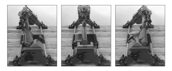
7. To rotate the firearm first release the spring-loaded knobs on both mounting bases. With the knobs released grab both of the assembly bases (be sure not to grab the mounting bases as they do not rotate) and rotate them together either forward or backward.
