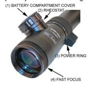
you are still able to see the reticle clearly. The "NV" position is designed for night vision use. The rheostat is located 45° left on top of the eyepiece. The battery, which is included with the scope, is a coin style CR2032 3V lithium battery. The battery can be replaced by first removing the battery compartment cover (1) located in the top of the rheostat adjustment (2), then remove the old battery, insert a new battery with "+" side facing up and retighten the cover (1).
