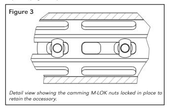
17. Removing the accessory requires 1 turn counterclockwise. The cammed nut will align with the recoil lugs on the accessory allowing the accessory to come off the rail. Care should be taken to not remove the nut from the bolt or M-LOK accessory. Loosening the screw further than 1 turn may result in permanent damage to the rail due to the issues described in **Step 17**.
