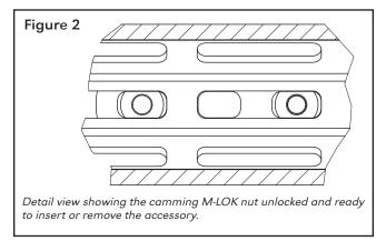
16. Begin to tighten the bolt one full turn with the hex key. The cammed nut will rotate, tighten, and eventually lock into place retaining the accessory on the handguard. Additional torque can be applied to hold the accessory in place (Figure 3).
