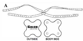
2. See Illustration B. Connect the holster to the harness: a right-handed shooter wears the holster under the left arm. Pay special attention to how the harness laces through the keeper. PRO TIP - to make adjustment easier, only thread the harness through the top and center loops of the swivel keeper temporarily - (see **Illustration C).** Do not install harness fasteners yet.
