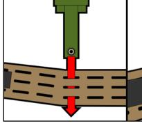
FEED MOLLE STRAP THROUGH OUTER BELT, IN TOP SLOT & OUT BOTTOM
