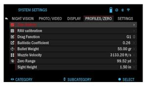
Open the Shortcut Carousel and navigate to Settings. Scroll to Profile/Zero and then select RAV calibration. You should see a velocity rating in the upper left corner (\_\_\_.\_\_ft/s or m/s) followed by "1, 2, 3". The First circle is blinking denoting actively searching for input. While having the RAV calibration active fire a round down range.
