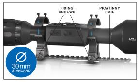
tion and mount the bottom portions of your rings to your rail for optimal eye relief. Place the scope on the bottom half of the rings you just mounted, verifying you have sufficient eye relief for your platform. Place the top portion of your ring over the mounted bottom portion, make sure the holes align and the screws turn easily. Apply equal torque to all screws with the provided Allen wrench. Make sure your rings are tight on your rifles rail and will not come loose due to recoil.
