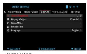
SCREEN BRIGHTNESS Gives you a 1 to 5 numerical selection, with 1 being the dimmest and 5 the brightest. It is recommended that you use the brightest setting during the day for optimal performance.
