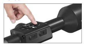
To TURN ON the device, press and hold the POWER button until you see the ATN splash screen.
