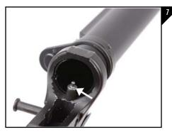
Next, screw the buffer tube into the lower until you come in contact with the buffer retainer pin and the buffer tube stops as seen in Figure 7.
