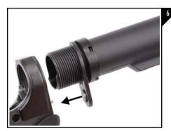
Place the lock plate onto the buffer tube making sure the extended end is facing towards the rifle as seen in Figure 6.
