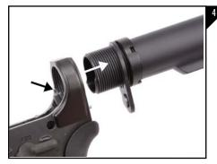
Using a punch, depress the buffer retainer pin and begin to unscrew the existing buffer tube. Once the tube clears the buffer retainer pin you may then finish unscrewing and remove hte buffer tube leaving the pin in place as seen in Figure 4.
