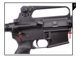
Reconnect the lower receiver to the upper receiver as seen in Figure 13 and push the rear and front take down pins back into place.
