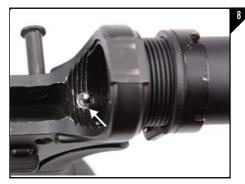
With your punch, depress the buffer retainer pin and make one more full rotation of the buffer tube until the buffer retainer pin sits into the groove on the buffer tube as seen in Figure 8. NOTE: For milspec installation there will be no groove on the tube, instead insure the tube covers the flat portion of the buffer retainer.
