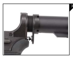
Next, using a AR tool, loosen the existing castle nut and slide the locking ring to the rear as seen in Figure 3 keeping in mind that the spring for the rear take down pin is under tension.
