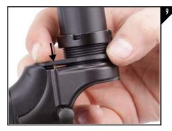
Press the locking ring tight to the lower receiver ensuring that the take down spring is properly seated as seen in Figure
