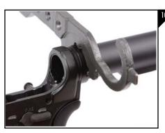
Hand tighten the castle nut to hold the locking ring in place. Then take the AR tool and tighten the castle nut until tight as seen in Figure 10.
