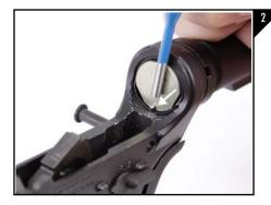
Using a punch, depress the buffer retainer pin as seen in Figure 2 and remove the buffer and spring. When removing, be careful as the spring is under heavy tension.
