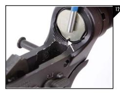
Make sure the spring is seated behind the buffer retainer pin as seen in Figure 12.
