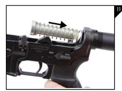
Reinstall the buffer and spring into the as seen in Figure 11.
