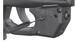
Screw down one of the provided battery door screws as shown with the mini Phillips head screwdriver in the tool kit.
